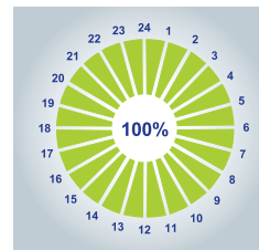
Fig. 11: If the circulation pump is operated continuously, the energy costs associated with provision of DHW equal 100 %.
